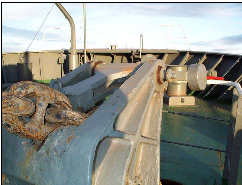
Fig. 15. Once the required amount of cable has been paid out, the vessel should be allowed to bring-up on the bow stopper. In any manoeuvring on the anchor the stopper should normally be engaged.
