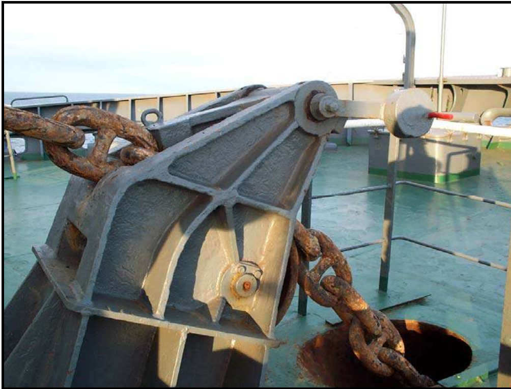
Fig. 14. The pawl, “guillotine stopper” form the integral part of the anchor cable restraining equipment and is designed to take the anchoring load.
